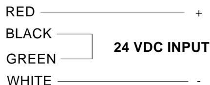
**Warning: Misconnection of wiring will cause the MOV surge suppression inside the electromagnetic lock to fail. This will not be covered under warranty.**
